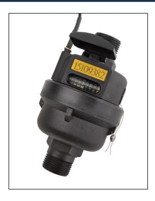
Carlon's vertical positive displacement<sub>®</sub> oscillating piston meter is designed for vertical installation but can be installed horizontally or on an incline provided the meter remains full of water. The meter has a built-in back flow preventer and is housed in an engineered plastic with is corrosion resistant liquid-sealed register for easy reading. The meter is available in gallons at 1 GPC (1 gallon per contact) or liters at 1LPC (1 liter per contact).
