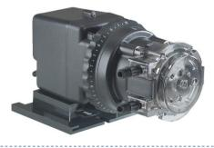
6 models up to 40 gpd @ 100 psi Flow rate output adjustment 5% to 100%, 2.5% increments Snap-fit design accesses three components without tools Inject at the well for disinfection and acidification. Wire pump into well pump circuit or pressure switch and manually adjust pump rate with external dial ring.
