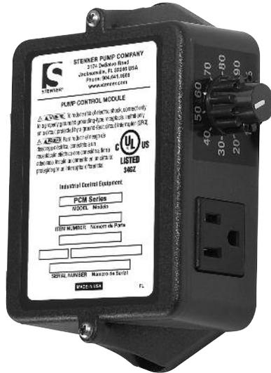
The Pump Control Module (PCM) is a time adjusted controller that powers the pump. A pulsing flow meter sends a signal to the PCM which actuates the pump to deliver the desired dose based upon water volume. The PCM has a locking feature on the adjustment knob.
