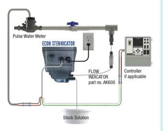
Wire a second Stennicator in series for system flows up to 5.4 gal/min.
