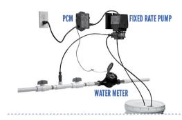
A pulsing dry contact water meter sends a signal to the PCM (time adjustable controller). The PCM actuates the fixed rate pump to proportionally inject the desired dose based on the system flow rate.
