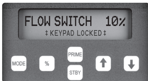
Example of control panel with keypad locked.
