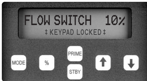
Example of control panel with keypad locked.
