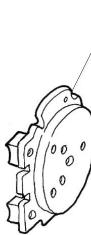
QP Tube Housing Cover with Leak Detect
